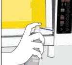
7. Lubricate Lubricate all the door bushings.
