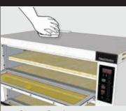
2. Clean Surfaces Clean stainless Steel front exterior, door handles, display, glass and shelves. Dry with a soft cloth!
