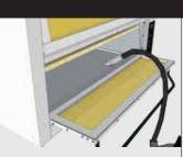
**10. Vacuum Oven Chamber** Vacuum the chamber and place back the stones exact in the same position and location.
