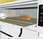
**3. Clean Stone** Brush and scrape out bake deposit or soot regularly during the day. Use a metal and soft brush!
